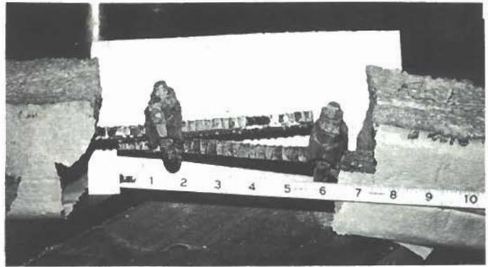
**FAILURE** of cable clamp splice.
