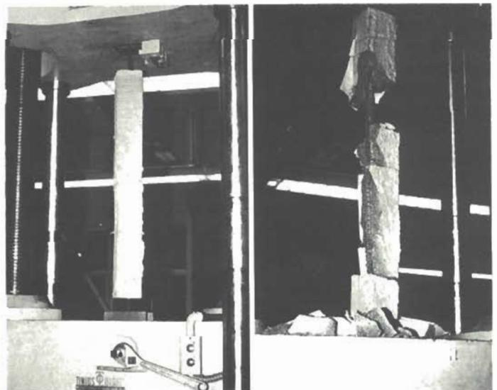
TESTING SPECIMEN (left) in tension in Tinius Olsen Universal Testing Machine. (Right) Failure of 24" lap splice.
