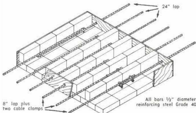
Casting jig of building brick which simulates construction conditions.
