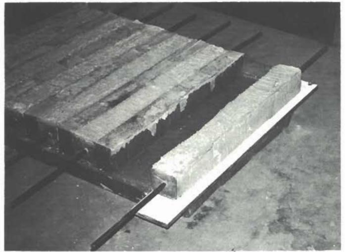
SPLICE SPECIMENS being removed from casting jig.
